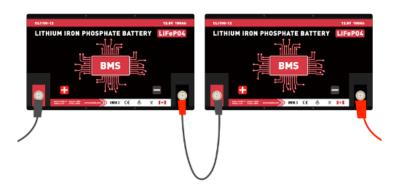
Connect up to 4 batteries in series or parallel
