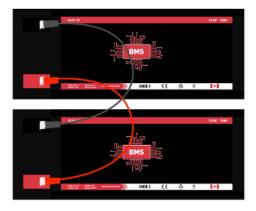
Connect up to 4 batteries in parallel or series
