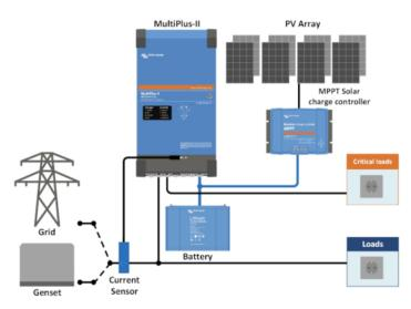
Grid parallel topology with MPPT solar charge controller The MultiPlus-II will use data from the external AC current sensor (must be ordered separately) or power meter to optimise selfconsumption and, if required, to prevent grid feed. In case of a power outage, the MultiPlus-II will continue to supply the critical loads
