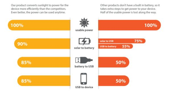
Using thin film solar cells has its advantages over standard crystalline cells. The LightSaver is able to capture power in much lower daylight levels than standard solar chargers. This means it starts charging earlier in the day, and later in the afternoon, and provides more useable energy over the course of any day of the year than any other solar charger in its power range.
